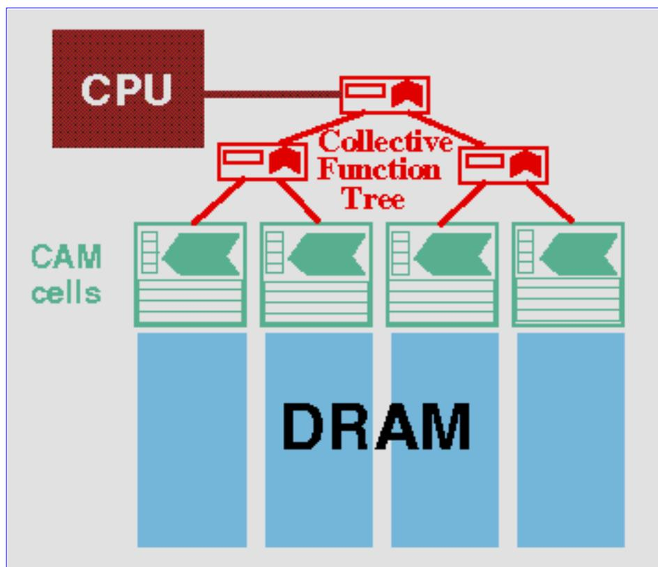
The [Rutgers CAM2000 Memory Architecture](#) uses the concepts of associative processing to overcome the shortcomings of conventional von Neumann machines in dealing with compute-bound applications involving massive amounts of data such as database mining. The architecture provides hardware support for data parallel, reduction, broadcast, and parallel prefix/suffix operations within a memory architecture that is DRAM compatible.
