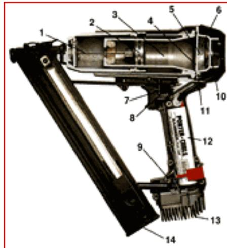
While [Porter Cable's Bammer](#) has nothing to do with Fuel Cells I thought it was an interesting application of a battery-free technology. A Piezo ignition system generates a spark causing a gas to expand to give an impulse to drive a nail.
